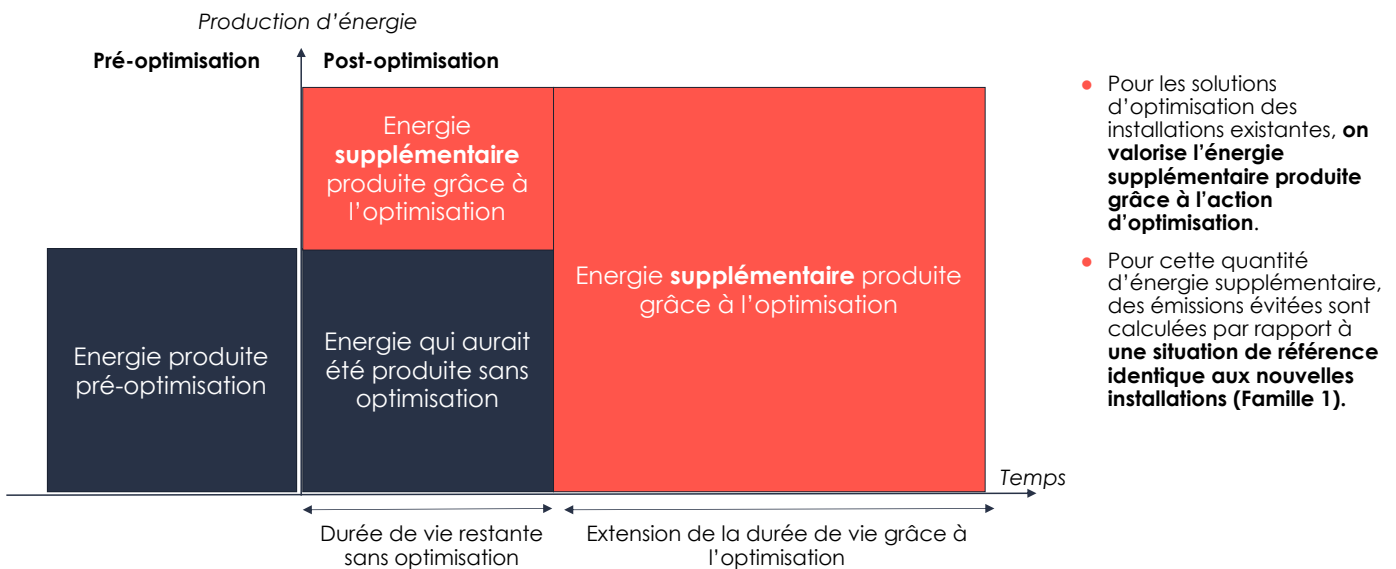
Illustration of the method for calculating avoided emissions by optimization solutions for existing facilities
